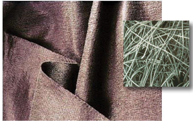
Figure 14. Non-woven needle punched geotextile with close-up
