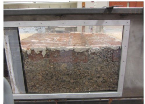
Laboratory flow testing device for University of Missouri PICP hydraulic research
